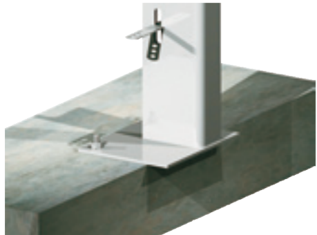
Base connection of an ACS "L" Type windpost fixed to the top of a concrete slab using chemical resin studs.
